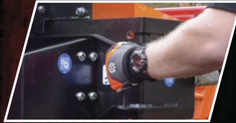
WolfPort Quick & easy access to the blades and rotor housing.
