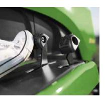
Intuitive Transmission Control: With these Side-by-Side Pedals, you can control direction and speed without raising a foot (not for the X106). The automotive-type accelerator control ensures easy operation, while the large pedal surface provides superior comfort during use. To adjust the height of cut, simply move the lever.
