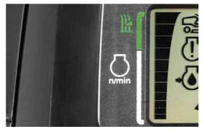
**Optimum "Best Cut" Target Zone:** The display shows you the optimum engine speed for outstanding cut quality. Always stay in the ultimate cut zone.
