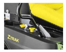
**Take Control:** The operator control panel is conveniently located and easy to use. It includes an hour meter, low fuel warning light, ignition switch, power take-off (PTO) control, and engine speed/choke control.
