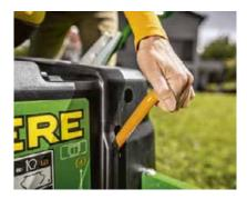
**Park Brake:** The park brake is conveniently located and highly effective at holding the machine in a parked position, even on sloped terrain.
