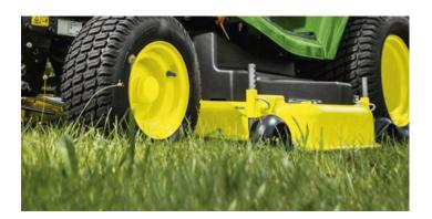
**The Accel Deep Mower Decks** deliver new levels of cut quality, productivity, cleanliness, durability and versatility: 4.5 in (11.4 cm) deep throughout the entire deck shell for optimum mowing, mulching and bagging performance. The stamped steel design eliminates sharp edges and corners where material can build up and diminish mowing performance.
