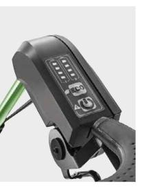
**Ergonomic Handlebar Design:** The handlebar can be height adjusted for improved grip comfort and grabbed in multiple ways to reduce upper body fatigue. Adjust the speed and check your battery status from the display, or engage eco mode for additional power savings.
