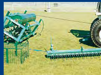
3 Drive tractor forward to roll Double-Quick over.
