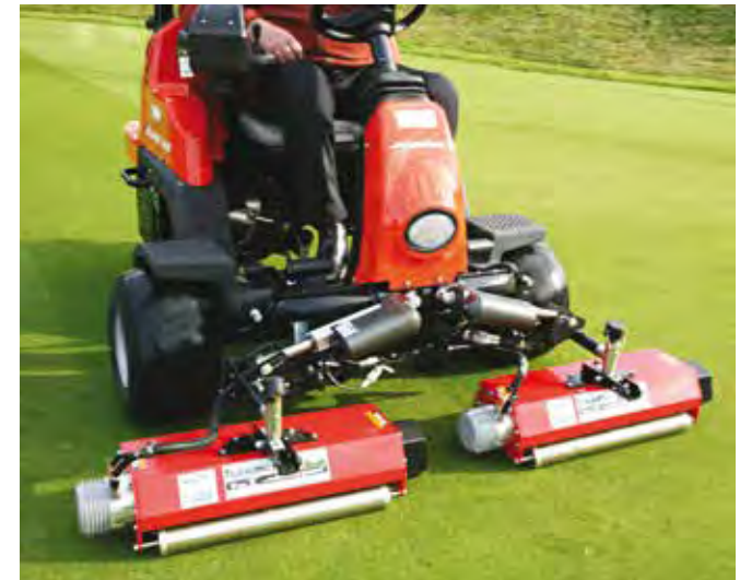
Select-A-Vibe rollers are available for both electric and hydraulic drive greens mowers.
