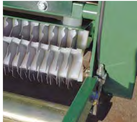
Tungsten tipped blades and finned spacers for ultimate cutting and collection performance.
