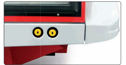
The exterior electric control for the front linkage is standard and makes mounting of attachments much easier.
