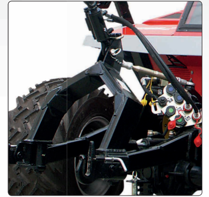
The Metrac H4 X has a front linkage with integrated lateral displacement as standard.
