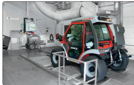
Before delivery, all vehicles undergo intensive functional testing such as here on the roller test bed (image).
