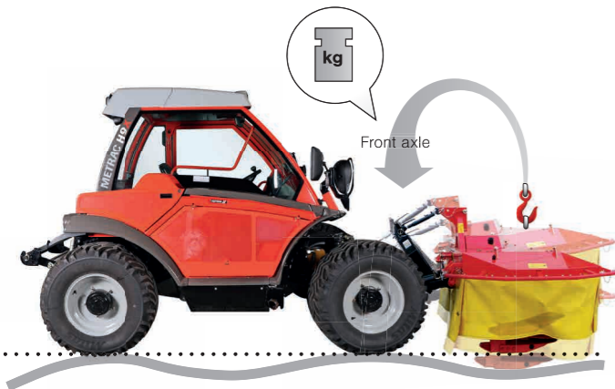
The mower follows the ground contours without changing the weight compensation pressure.
